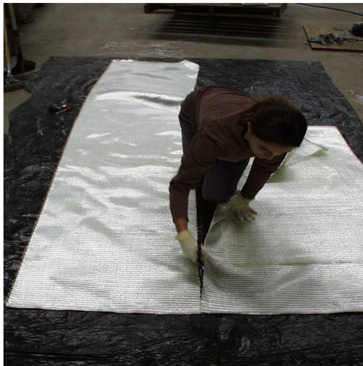
Figure 6.1 Cutting the fabric
