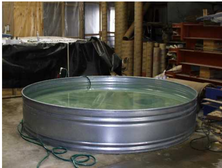
Figure 7.1 Storage Tank Filled with Salt Water
