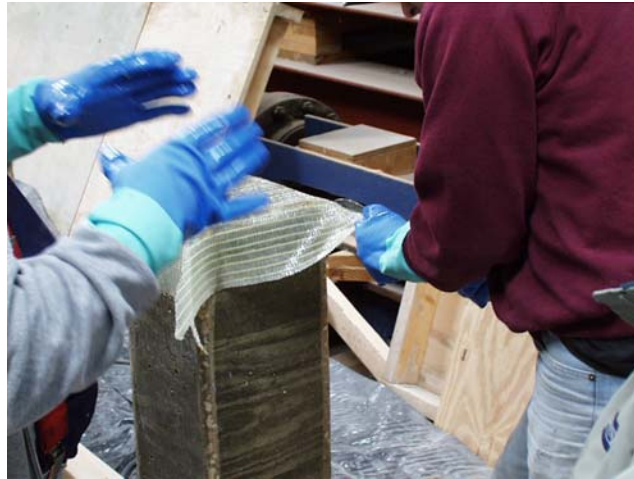
Figure 6.3 Wrapping A Beam End
