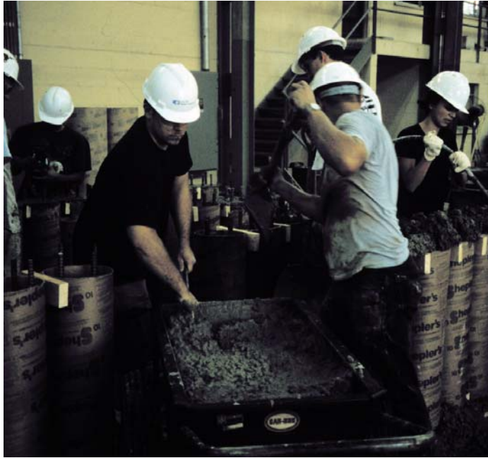
Figure 5.3 Placing Concrete in Cylindrical Forms
